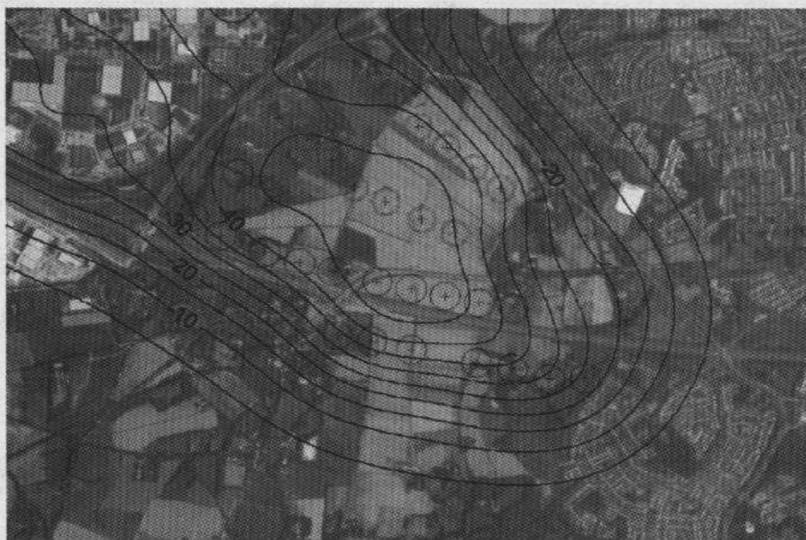
Figure 10: Cavern field layout and subsidence prediction in mm/100 years
